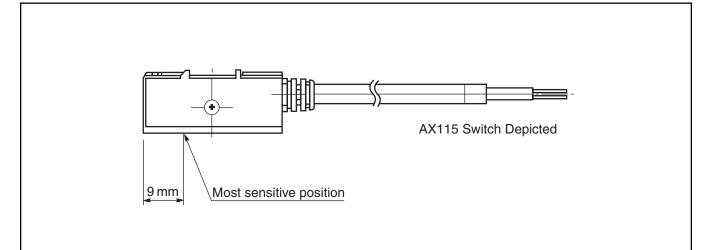
The most sensitive position of both switches is located 9mm from the end. When the piston magnet is placed in the ideal adjustment range, the indicating lamp lights green. For the
