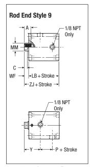
20 and 25mm Bore Series CHH Port Detail 5 and 10mm strokes only
