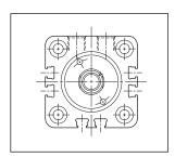
20 and 25mm Groove Detail (CHH has no grooves.)
