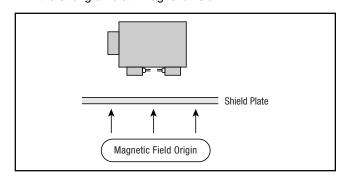
Do not bring the strong magnetic bodies (iron, etc.) near the cylinder body and switch. As a rule, such materials shall be kept over 10mm from the switch.
