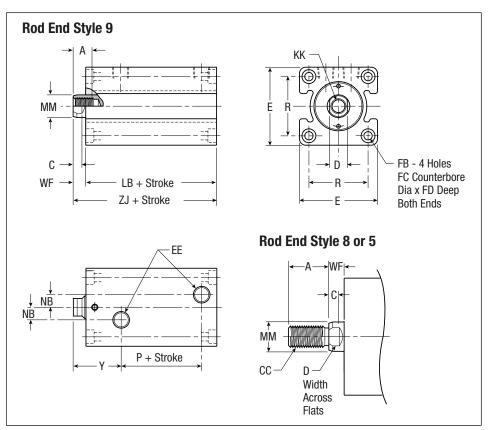
32 through 100mm Bore - Series CHL with Switch Grooves
