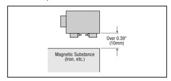
The interval shall be kept over 15mm when multiple switch-set cylinders are used adjacently. Switches may perceive the magnet of the above cylinder inadvertently.
