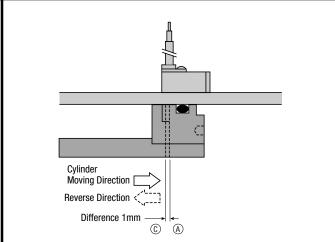
When the piston reaches position "A" and then returns in the reverse direction <, the switch remains on until the piston reaches "C." The interval between "A" and "C" is called the difference.
