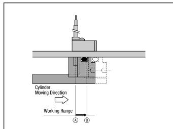
When the piston moves in the > direction and the magnet arrives at position "A," the reed switch actuates. The switch remains on from "A" to "B." This is called the working range.
