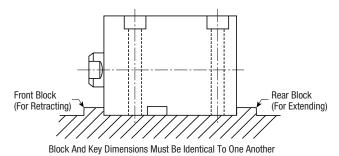
When installing a cylinder without a key, be sure to place blocks at each end. Bolts alone may not support the cylinder's force, which could result in damage to the bolts.
