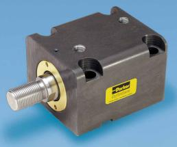
SAE Ports available on 32 - 100mm bores One-piece, Extruded Cylinder Body Hard Chrome Plated Piston Rod Precision bored with no end cap Magnetic Piston Option High Strength Bronze Rod (CHL only) for reed or Bushing for reliable service hall effect proximity sensors Available in male and Corrosion Resistant Exterior female rod ends Aluminum Alloy (CHL) Black Oxide Steel (CHH)
